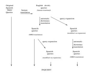
Figure 1: Flow chart of query processing.
