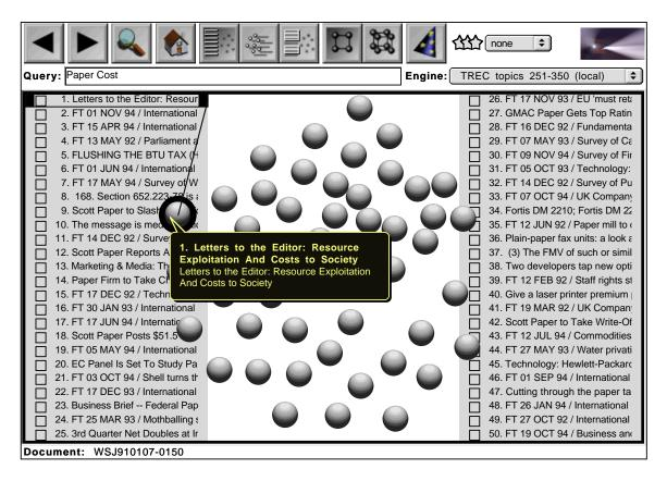
**Figure 5.2.** Screen shot of the system that integrates the spring-embedding visualization and the ranked list. The top fifty documents retrieved by the INQUERY search engine for the "Paper Cost" query. A two-dimensional picture is shown.
