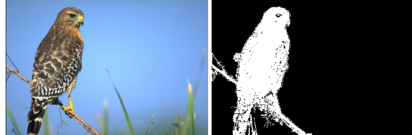
Figure 9: Example showing partial elimination of background where the included background does not affect the color distribution of the final segment significantly.
