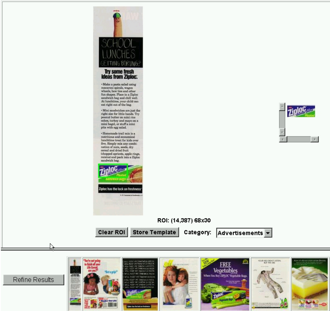
Figure 3.14. Online user interface to FOCUS showing a query box being selected and the results after first phase of processing (where the first, third and fifth images contain the query object)
