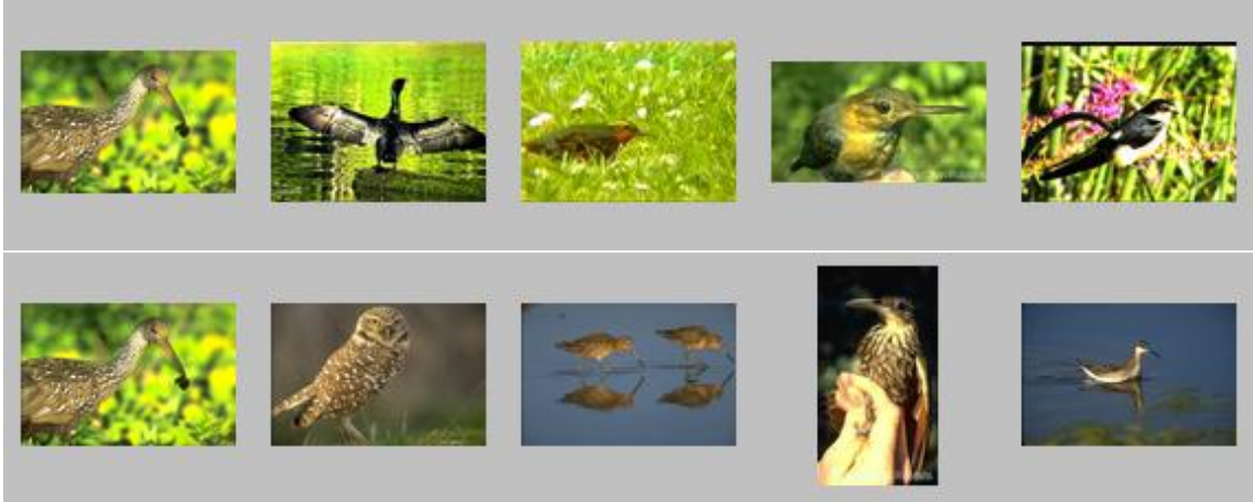
Figure 5.2. Qualitative improvement in retrieval obtained when only the bird region is used for indexing. The query is the leftmost image. (top) whole image color-based retrieval (bottom) retrieval after indexing only the colors from the object of interest found by the method described in this chapter
